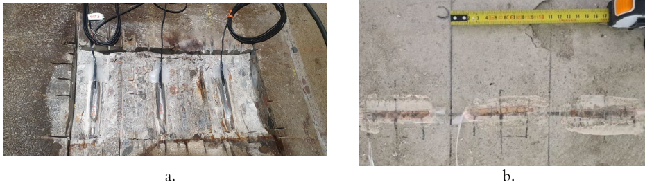
Figure 23. Instrumentation for a. strain cut and b. saw cut methods.
